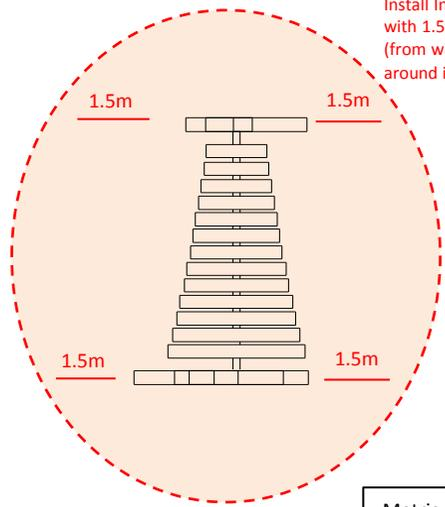
Install Instrument with 1.5m free space (from widest point) around it.
